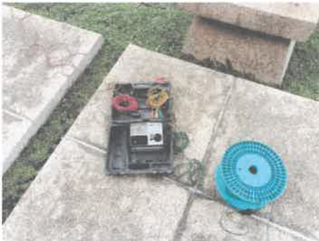
Preventive maintenance Ground resistance test.
